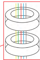
Port sieciowy AC, GRID-L1, GRID-L2, GRID-L3, GRID-N, PE (dla EMC)
