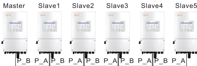
Figure 3.24 Parallel Terminal Connection
