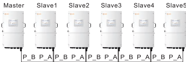
Figure 3.23 Parallel Terminal Connection
