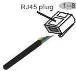
Figure 4.36 Strip the insulation layer and connect to RJ45 plug
